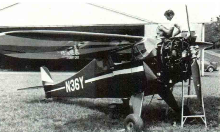
John pours in some petrol preparatory to firing up the engine for the first time since overhaul. The 23 ft. one piece wing supports itself quite well without struts.
