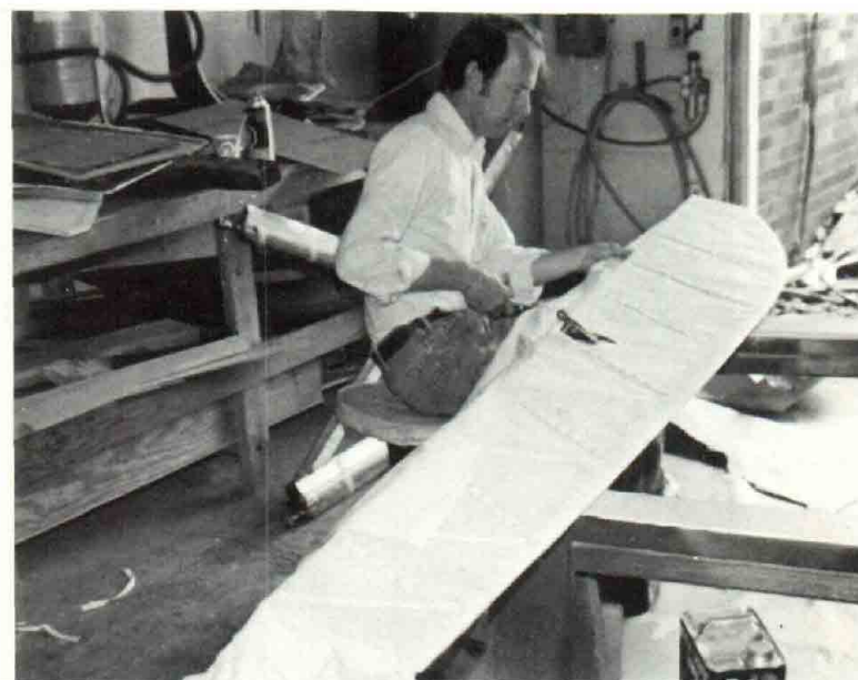
Ken Hyde (EAA 37179), RFD 1, Warrenton, Va. 22186 applying fabric to one of the ailerons. Ken is one of the nation's super restorers of antique aircraft.
