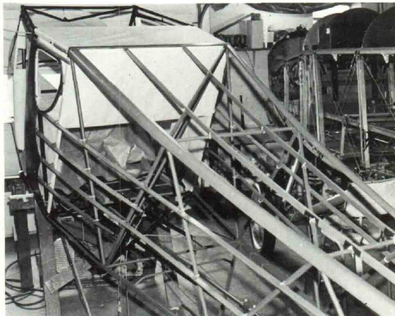
Here is how Monocoupes get those nicely rounded fuselage corners — a lot of woodwork. That's one of Ken Hyde's Curtiss Jennies on the right.
