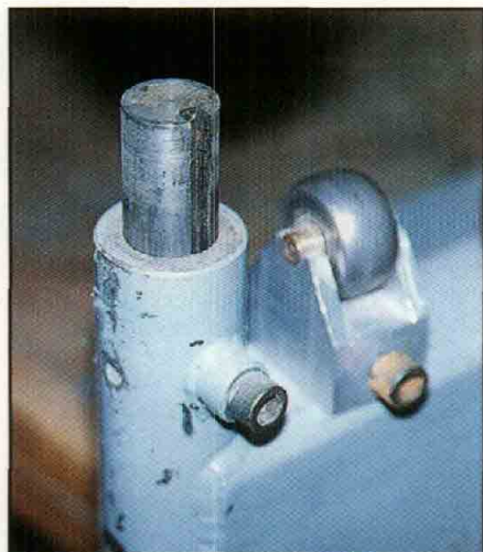
The welded boss provides enough wall thickness to accept the stop-bolt threads.
