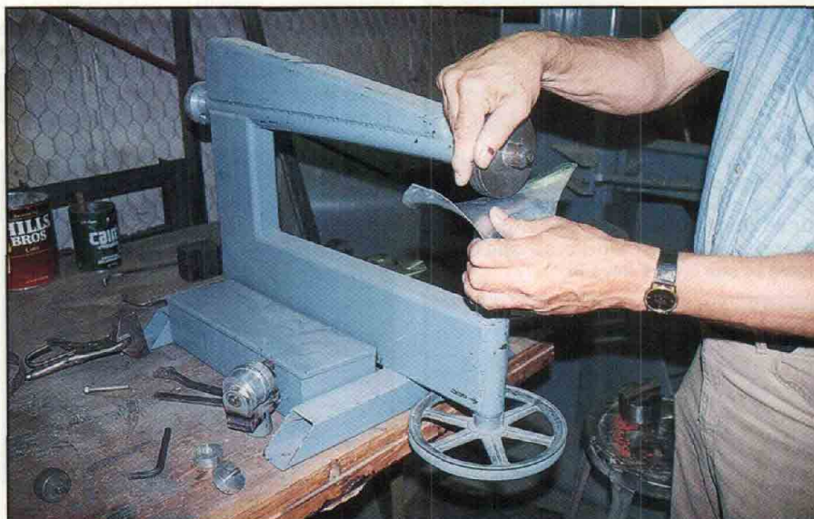
Using the baby wheel differs from the large one in that the upper wheel is driven by the operator's free hand rather than trying to push the work piece through the rollers. If working on a larger piece it can be pushed, but it isn't necessary. The small size of the rollers lets the little wheel work in really small radii, but there's nothing stopping a homebuilder from substituting larger rollers for larger work.
