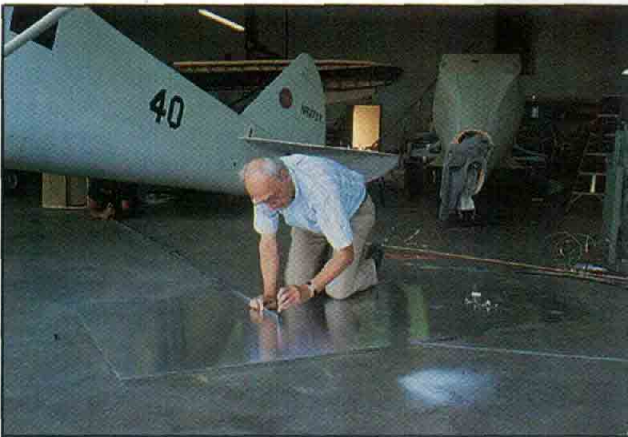
The skirt radii were so long a giant compass was made from aluminum angle. If you look carefully you'll see Bob Bell under the Mulligan fuselage establishing the center point while Jim swings the arcs.
