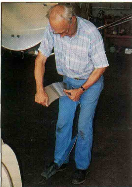
The first forming operation for the nose section is pretty rudimentary using tools most builders have in their shops.
