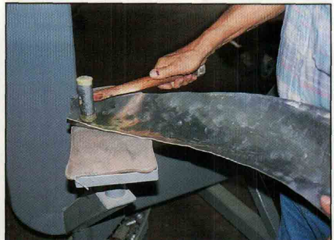
Because there is so much stretching on the nose section, it is first hammered down into the shot bag. No finesse is required since the goal is to stretch the metal, not form or shape it.
