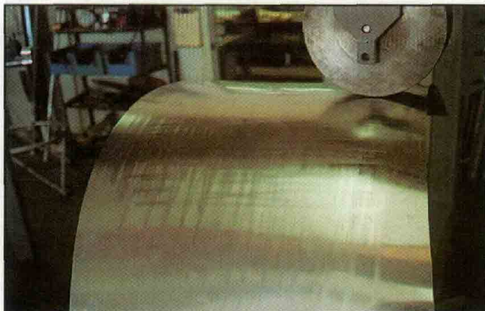
The crisscross pattern of the roller marks show where Younkin has been dividing up his rolling so the compound curve develops without radically changing the radius of the skirt.
