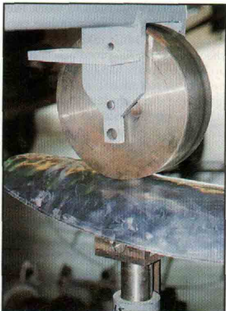
Initially the English Wheel is used to flatten out the hammer marks but, as work progresses, it will be doing its own stretching. This smoothing process could have been done by hand, but the wheel works much faster.
