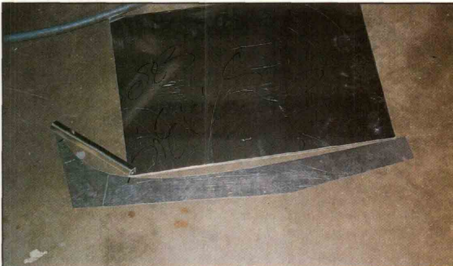
The white template represents the cowl outline with the bumps in it to clear the rocker arm boxes. The two black marks are the edges of the front cowl section. The aluminum template is the surface line of the cowl without the bumps which lies down between the rocker arms.
