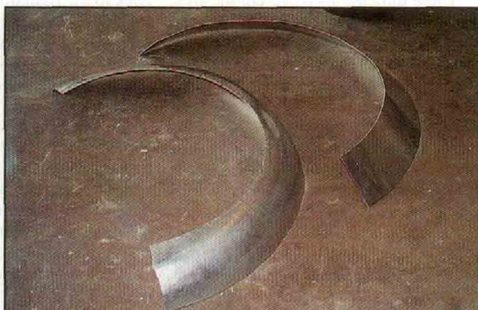
Before and after. Total time invested is less than an hour. By the time all the rolling and hammering had been done, the relatively soft 3003 H-14 aluminum has work hardened considerably. The ends will be trimmed on assembly.
