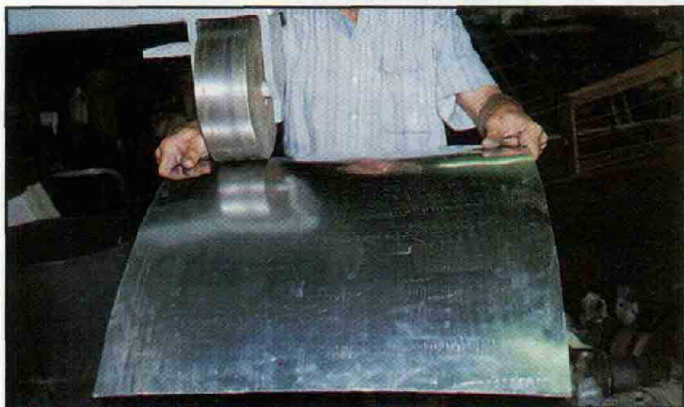
The skirt was so large and the curve so gentle it didn't require using the shot bag for the initial stretching. Stretching it on the wheel was much more gradual although Jim preferred using the power hammer.
