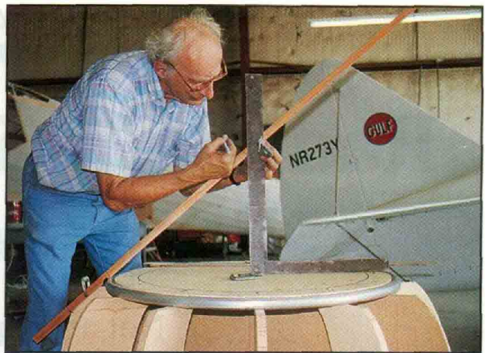
Jim Younkin uses straight edges and a tape measure to layout the geometry necessary to determine the pattern radii.
