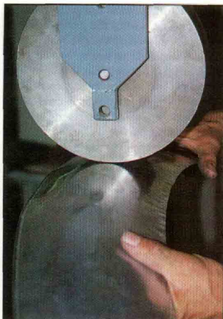
Only about 15 minutes separates this picture from the last one. The Wheel does its work very quickly. Here it is being used crosswise to keep the radii of the part from shortening.
