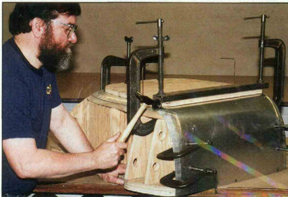
With everything clamped tight, the metal is tapped down to meet the MDF form.
