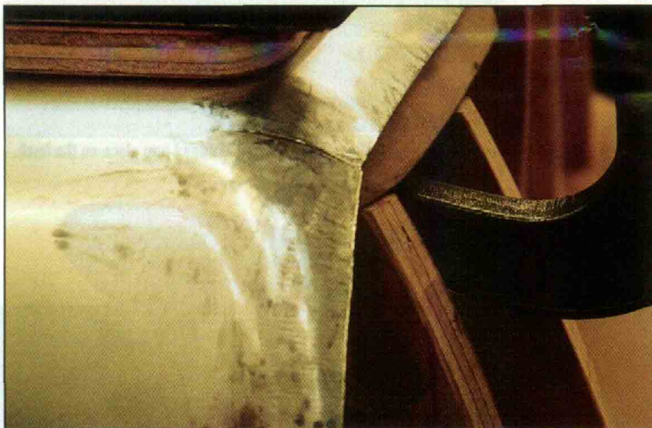
Here's a close-up shot of the corner — the area where the greatest shrinking was required. Notice that a small relief was cut to ease the shaping in this area.
