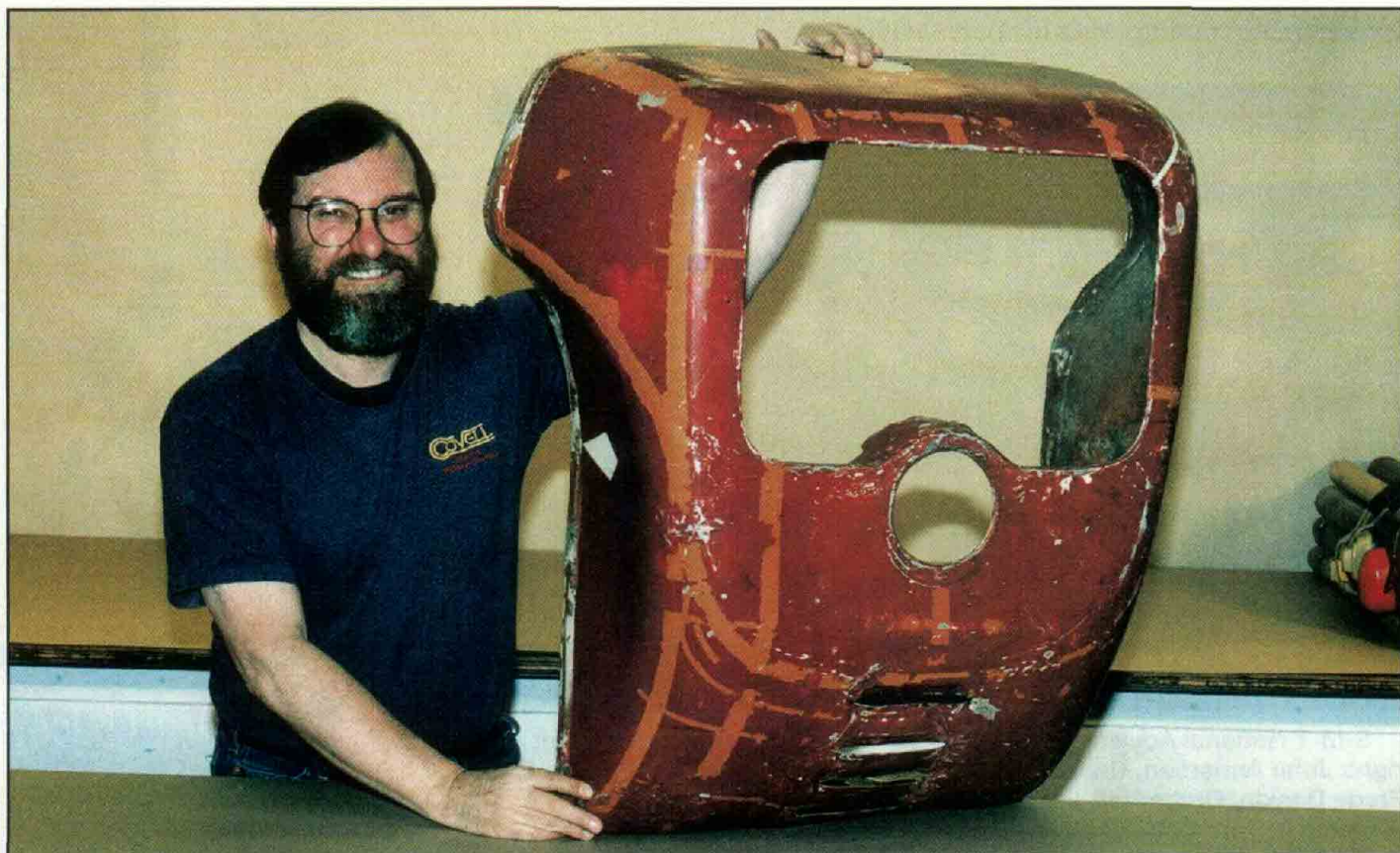
The author Ron Covell holds an original Curtiss-Robin nose bowl, graciously lent to us by Dick Fischer to use as a pattern for creating a copy for Alan Holloway's restoration project.
