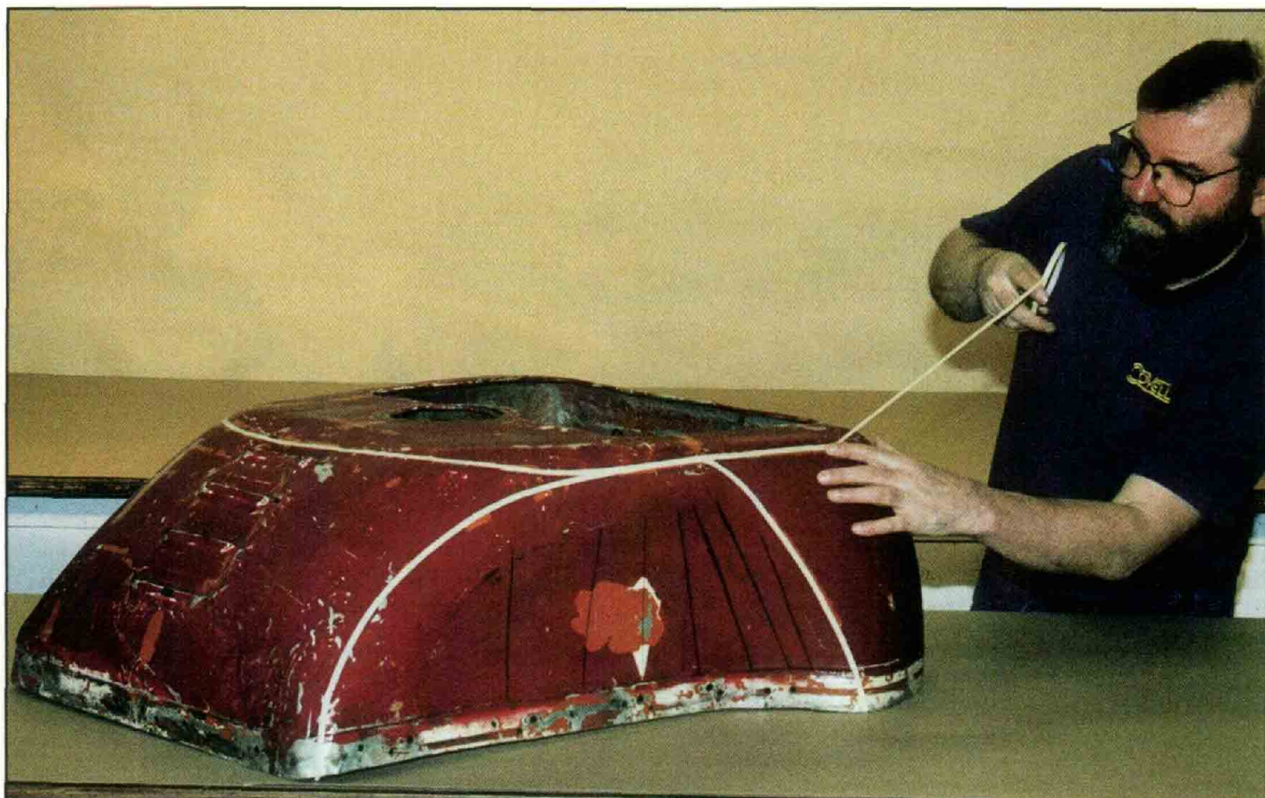
We're using 1/4" masking tape here to plot where the joints between panels will be placed. The process used for shaping the metal has a lot to do with where the joints are positioned (see text).
