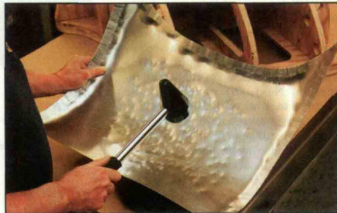
The center portion of the panel is bulged slightly with a mallet and sandbag.
