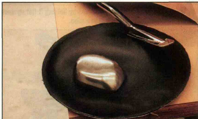
For planishing the shape smooth, we're using a slap hammer and dolly with a low crown face. Notice how we've supported the dolly with a sandbag, so we have a free hand to hold the panel.
