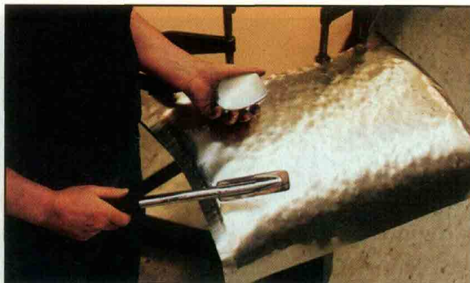
We're ready to planish the panel smooth. Notice how the panel is clamped to the corner of the workbench, freeing up our hands to use the slap hammer and dolly.
