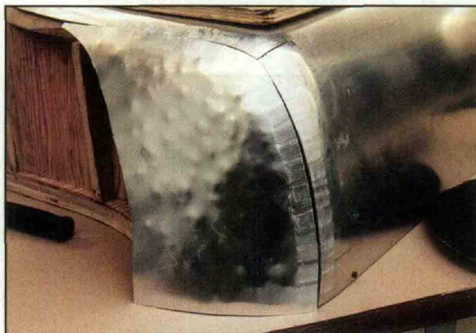
The rough-shaped panel is test-fitted against the buck.
