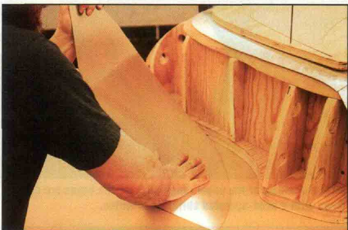
The lower side piece is shaped freehand by holding it flat against the workbench, and gently lifting one edge.
