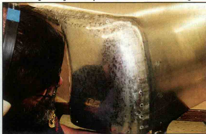
Using a hammer and dolly to work the seam for perfect alignment of the edges.
