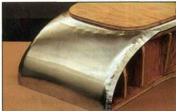
Test-fitting on the buck again. Notice how much shape has been put into the panel just by using the shrinker!
