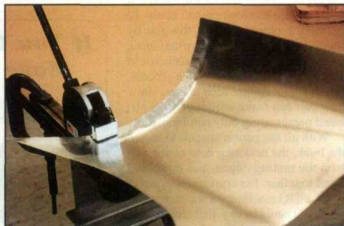
Using a hand shrinking machine to pull the edges down.
