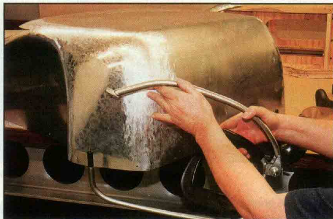
This is a "Bullseye Pick," used for gently tapping up the low spots.
