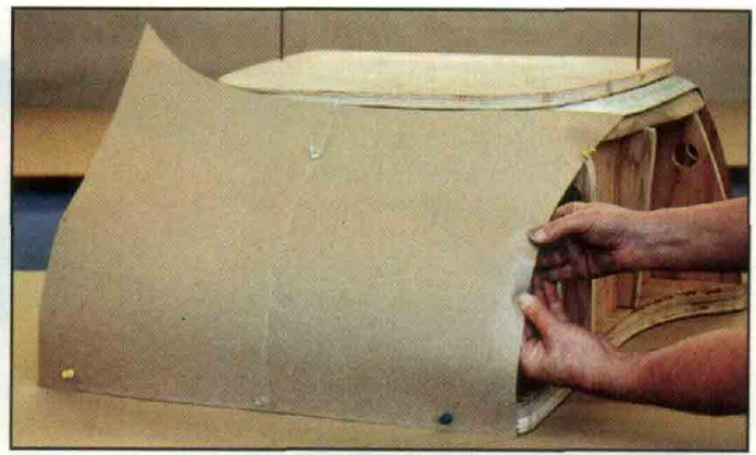
Using chip board to make a pattern for the bottom piece. Note the use of push pins to anchor the board to the buck.
