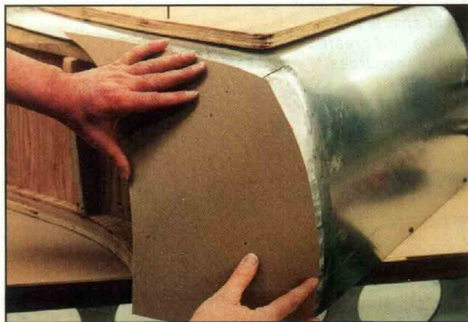
We're using chip board as a material to make the pattern for the upper side portion of the nose bowl, allowing a 1/2" overlap.
