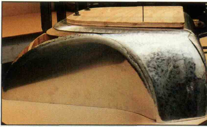
Another test fitting on the buck, paying attention to how the contours of the panels match.
