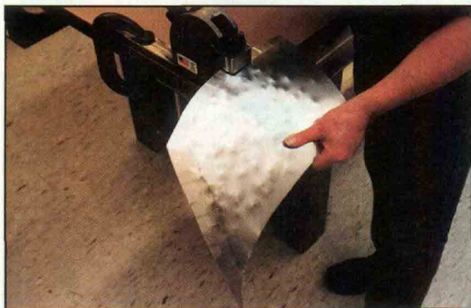
With the middle of the panel rough-shaped, the edges are drawn down with a hand-operated shrinking machine.
