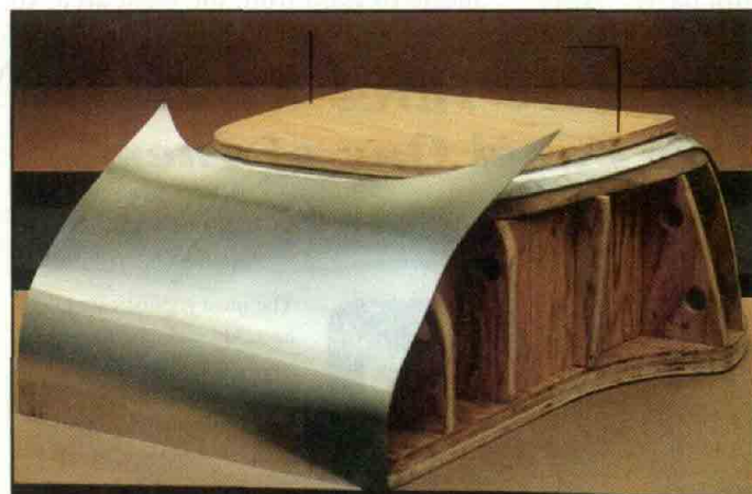
The first fitting on the buck, after the profile is shaped by hand.
