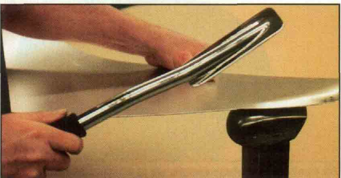
The edge of this panel is rounded over using the slap hammer and post dolly.
