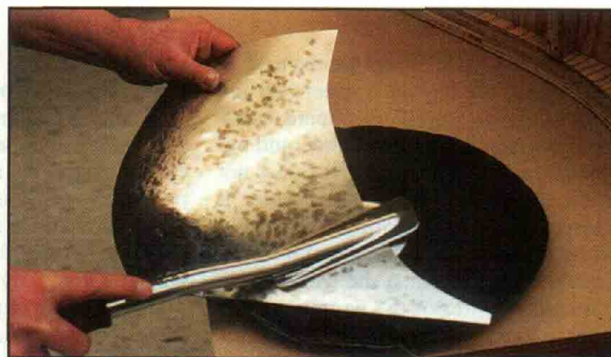
The planishing nears completion. It took about five minutes to planish this panel smooth.
