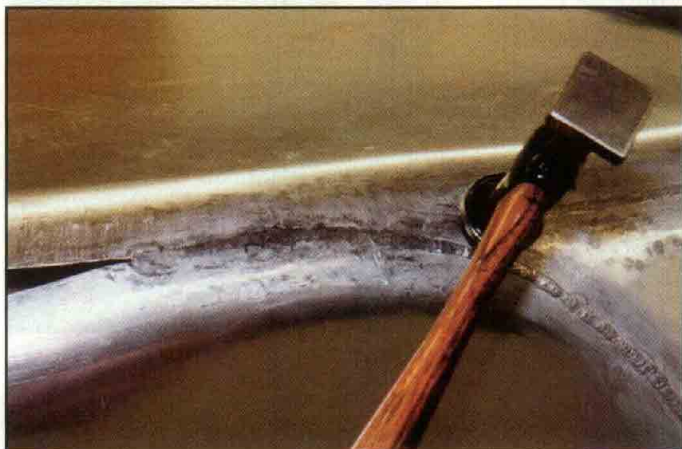
Using a hammer and dolly to planish the welds down flat.
