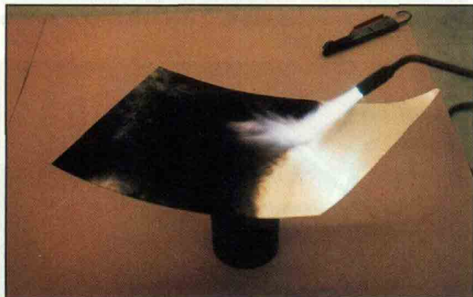
After the panel is cut out, it is annealed with an oxy-acetylene torch.
