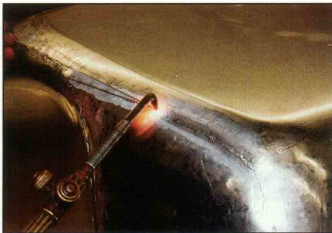
We're welding the seam with an oxy-acetylene torch.
