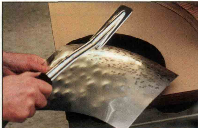
In this shot, you'll see that about 1/4 of the panel is planished. This took about one minute.
