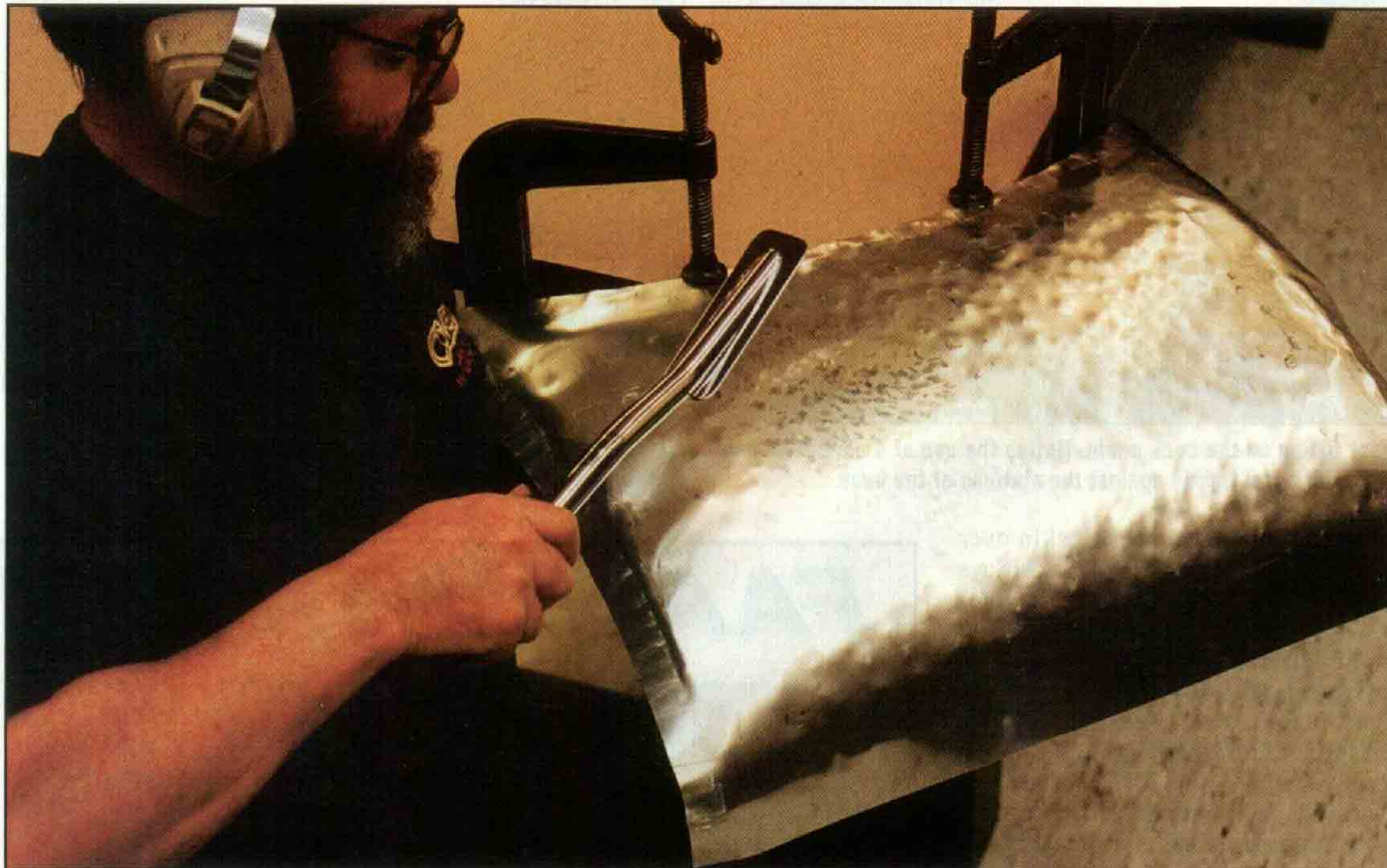
Here you can see the relative smoothness of the planished area compared to the rough-shaped areas.
