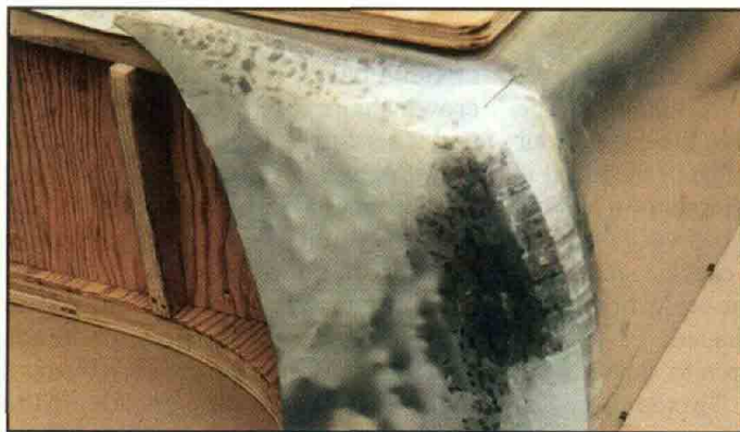
The panel is test-fitted to the buck to test its shape as the planishing progresses.
