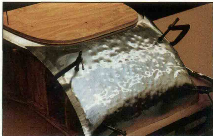
Test fitting on the buck again. Notice the use of C clamps to help hold the panel tightly against the stations of the buck.
