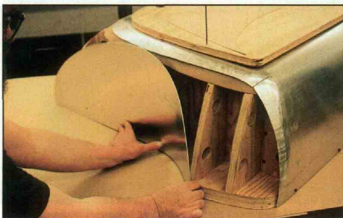
After a few adjustments, it fits the buck very well.
