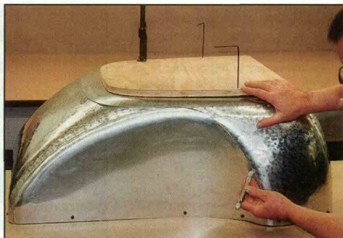
Scribing the edge of one panel onto another for trimming.
