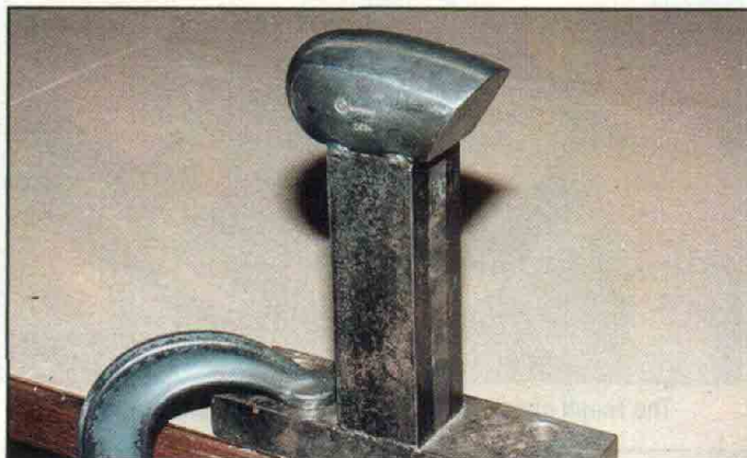
This is a shop-made post dolly, created by welding a dolly onto a shop made support.
