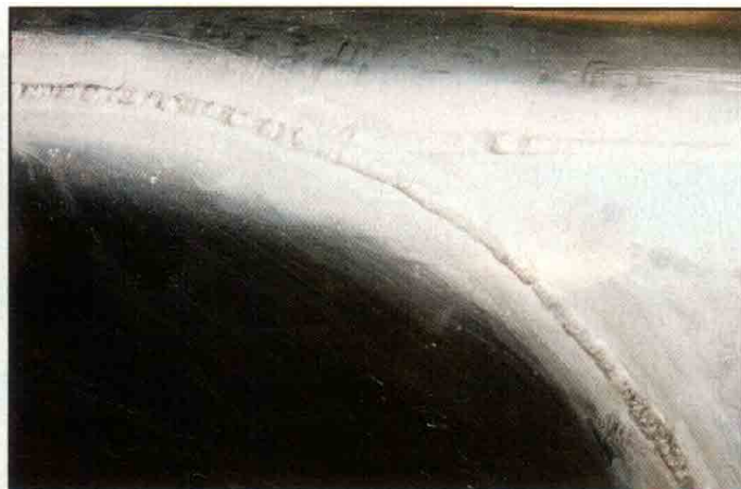
A close-up look at the welded seams. Note the consistency of the weld heads.
