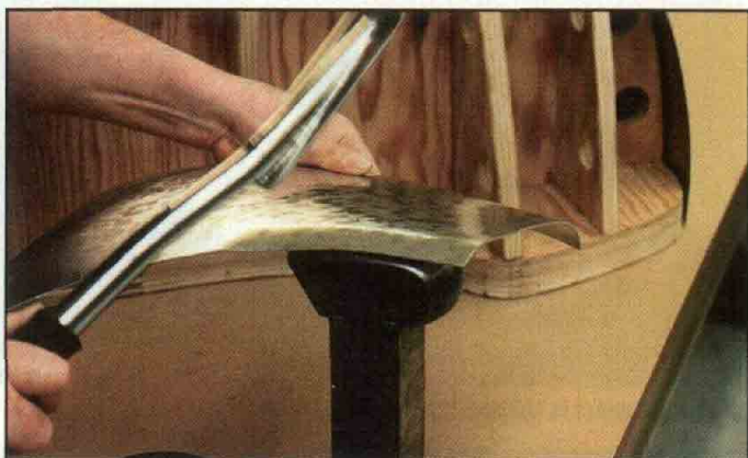
We're using the post dolly and slap hammer to round over the edges of the panel.
