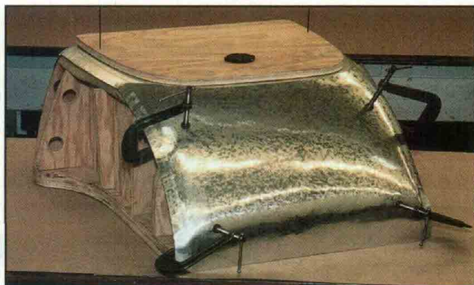
With this panel completely planished, you can see how well it matches the contour of the buck, and how smoothly it blends in with the other panels.
