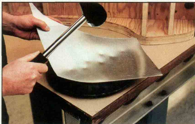
The rough shaping is done with a mallet and sandbag.
